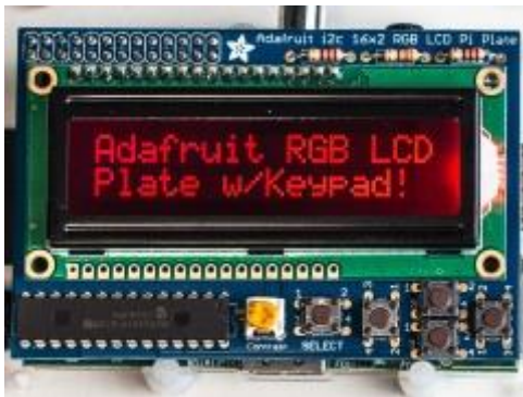
i2c 16x2 LCD display + 5 key keypad
